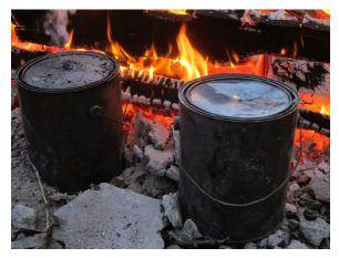
When the flame starts to diminish keep a good eye on the canister: the moment it goes out, remove the can from the fire and plug the hole.
