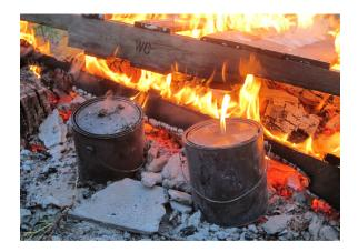
After a long time, the smoke will start to peter out, as you can see at the left canister. Do not mess with the can as now it is time for the flame to appear. Make sure the fire is well built at this point to help the combustible gasses to ignite.
