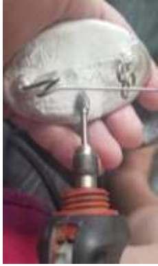
Removing some material to reduce weight.
