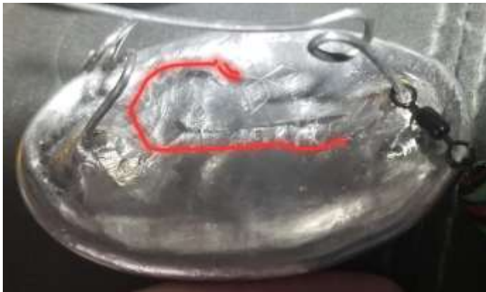
The red “J” showing the imbedded pin starting to show though the pewter.
